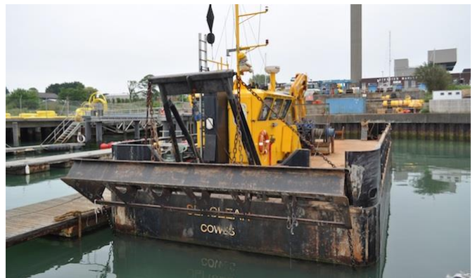
Figure 15 (right) - Cowes Harbour Commission using multicat fitted with a box plough
