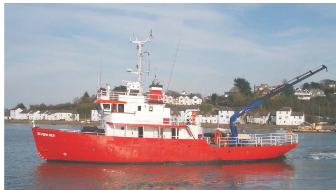
Figure 26 – examples of vessels expected to operate at Wave Hub during installation and operation and maintenance phases of wave energy device deployment. Left – Green Marine’s Green Isle Damen Multi Cat 2712 – 27.7m length and 2.85m draught. Right – KML’s Severn Sea support vessel - 30m length and 2.5m draught.
