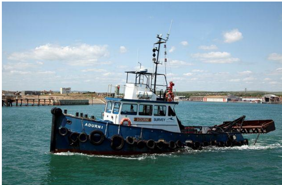
Figure 17 – Damen 1405 tug used for plough dredging at Shoreham Harbour
