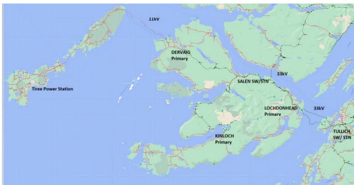
Figure 10 Existing network infrastructure in Mull and Tiree
